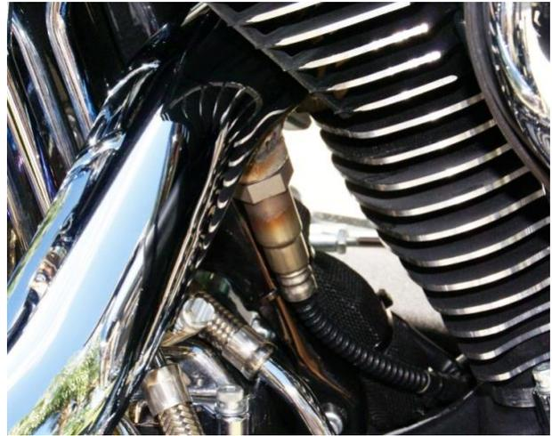
Typical Rear Sensor Installation
