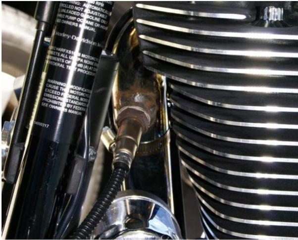
Typical Front Sensor Installation
