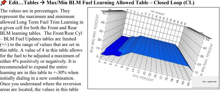
should be reduced to lower values. Typically 4 in reversion areas, 10 at lower throttle openings, 20 in the midrange and 15 at WOT.
