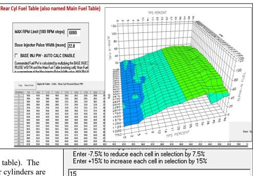
Cyl - BLM Fuel Updates [Block Learn Multiplier]) to arrive at the corrected injector pulse width. The correction is applied based on the information learned by the wideband oxygen sensor signal.
