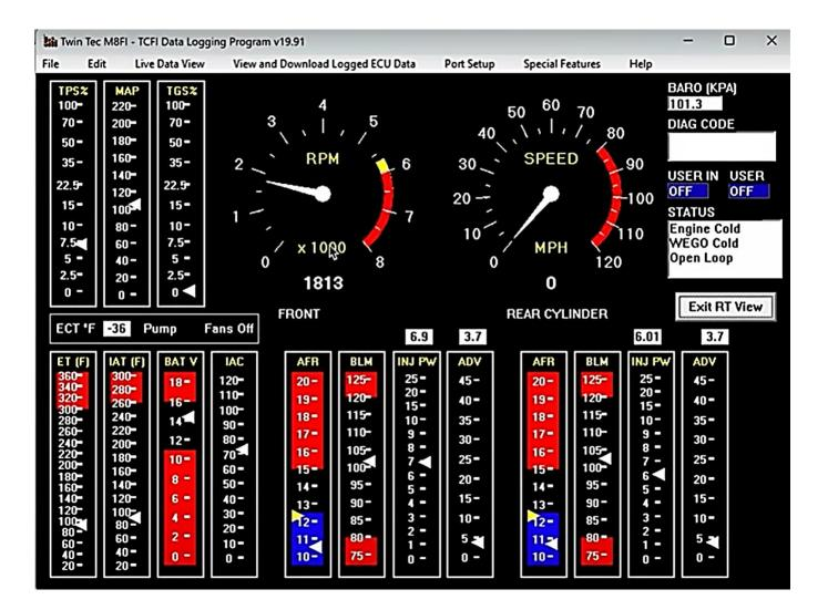
Real time engine data is displayed on an instrument panel type layout with round tach and speedometer gauges and bar graph type gauges for most other parameters. Barometric pressure, any diagnostic codes, status of the user input and output, and status messages are displayed in additional windows. If the engine is not running most values will appear as zero.
