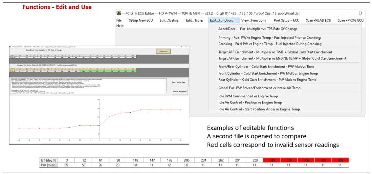
You can edit the numeric data corresponding to the dependent variable on the lower row of the spreadsheet grid. A typical 2D table is shown. Some of the engine temperature cells are highlighted in red. These red cells correspond to extreme sensor readings. After you have edited the table, you must click **Save Update Data** to save your changes into memory.
