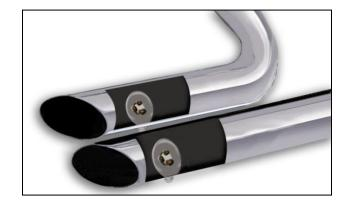
**Excessive scavenging**. Tuned exhausts in combination with a high overlap camshaft profile can pull unburned air and fuel mixture through the cylinder into the exhaust and cause an erroneous rich AFR indication. Some aftermarket 2-into-1 systems, such as the Thunderheader appear to suffer from this problem, whereas others such as the Supertrapp seem less affected.
