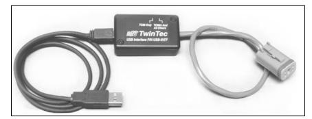
terminal Deutsch data link connector that is part of the WEGO harness. The USB Interface has a switch that selects the operating mode. For communication with the TCFI, you must use the **TC88A And All Others** switch position.
