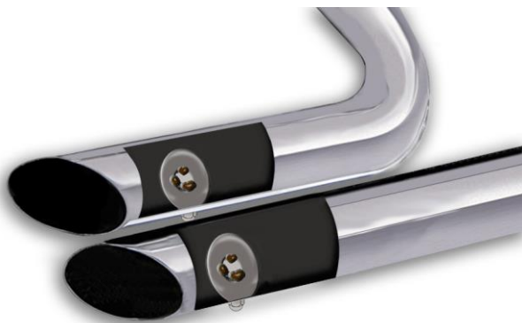
Figure 1 – Exhaust Mod to Reduce Reversion
