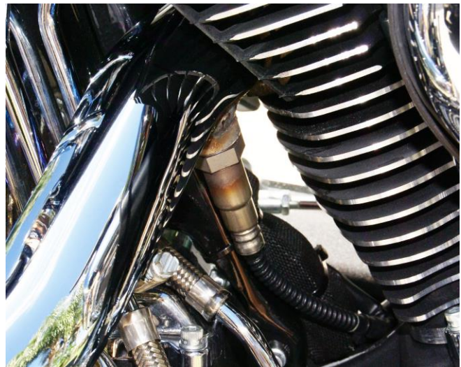
Figure 25 – Typical Rear Sensor Installation
