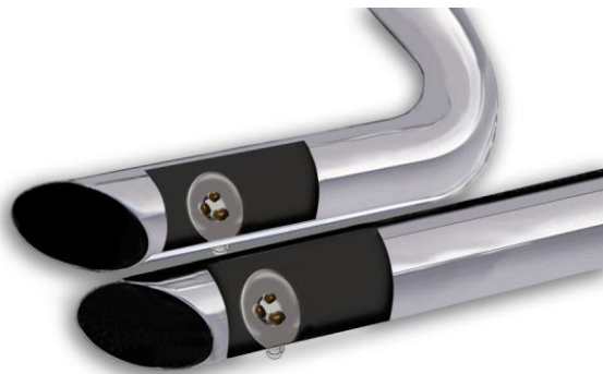
Figure 1 – Exhaust Mod to Reduce Reversion
