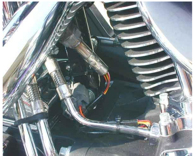
Figure 26 – Typical Sensor Installation
