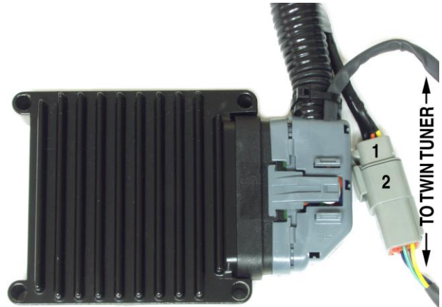
Figure 5 – Completed Wiring at ECM
