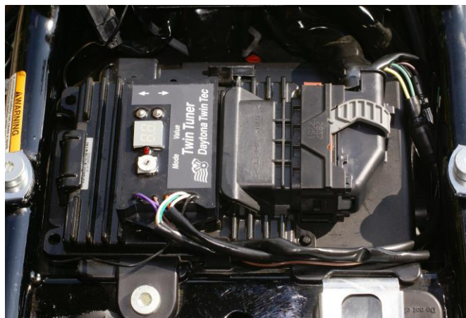
Figure 8 – Completed Twin Tuner Installation
