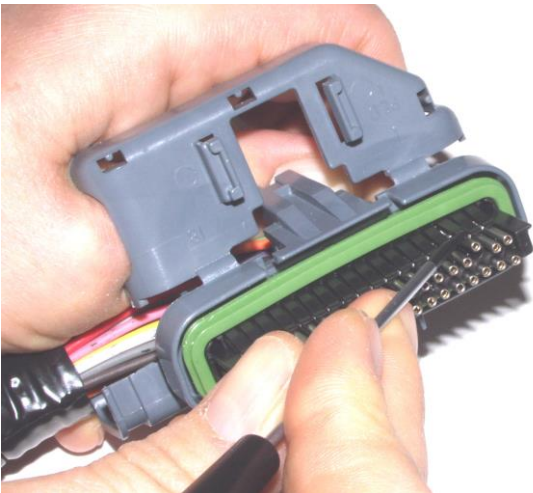
Figure 4 – ECM Connector Terminal Removal
