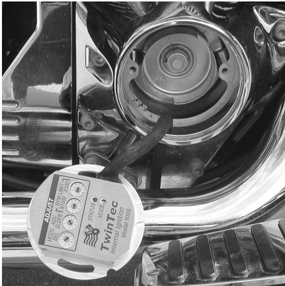
Figure 1 - Feeding Harness Thru Exit Hole
