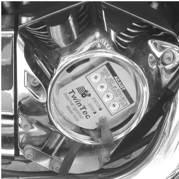
Figure 2 - Installing Unit (Note Orientation)
